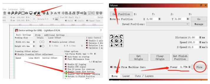
3. How to position laser engraving? <u>suggest: Fire laser light 0.75% power—Center the axis of object and the laser —Framing to preview engraving position</u>
