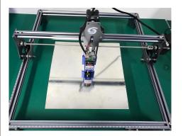
Before each engraving image, Move the laser to the middle of the frame.
