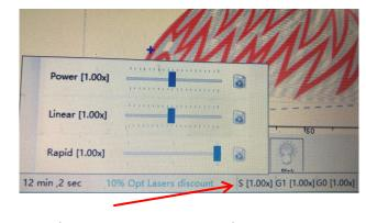
laser Power,Linear,Speed adjustment
